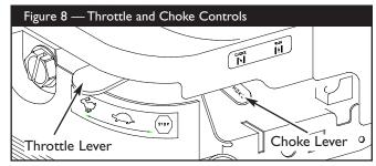
Move the choke lever to the "Choke" position (Figure 8).
