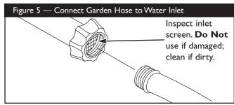
Run water through your garden hose for 30 seconds to clean out any debris.
