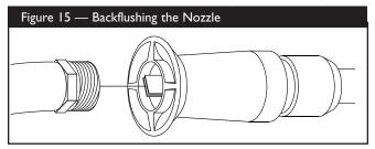
Reinstall the nozzle and in-line filter into the nozzle extension. Do Not overtighten the nozzle with the allen wrench.
