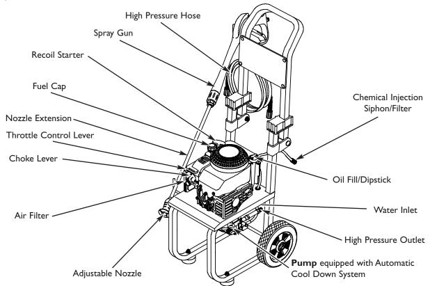
**Adjustable Nozzle** — Always attached to nozzle extension. Adjustable nozzle allows you to adjust spray pressure and spray pattern.
